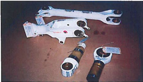
Figura 8 - side brace lower - upper, rod end, bolt axle wheel MLG e crank semilavorati (mock-up)
